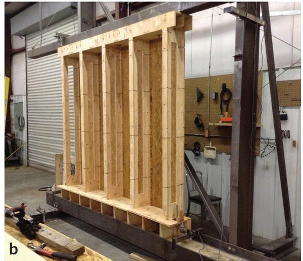
△ Figure 10. (a) Racking test diagram showing sensor locations; (b) racking test. Drawing and photograph by Michael Stoner. Reproduced with permission.
