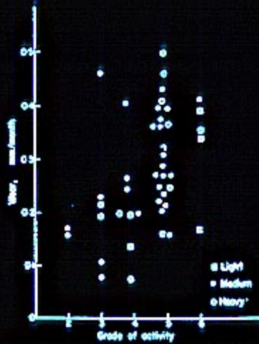
FIG. 4. Plot representing patients of different weight in relation to the rate of wear and the grade of functional activity of each case.
