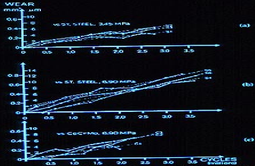
Fig. 6. Wear of UHMW polyethylene as a function of sliding distance (one cycle = 50 mm) using serum lubrication and highly polished counterfaces. (a) 316 stainless steel at 3.45 MPa, (b) 316 stainless steel at 6.90 MPa, (c) cobalt-chrome alloy at 6.90 MPa. The dashed lines are the best-fit straight lines for each set of data, calculated using linear regression. The slope of this line is the wear rate for each specimen (Table III).
