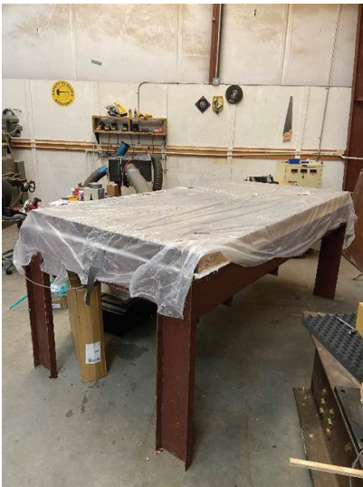
Figure 1. Pressure chamber for cyclic pressure/suction loading test
