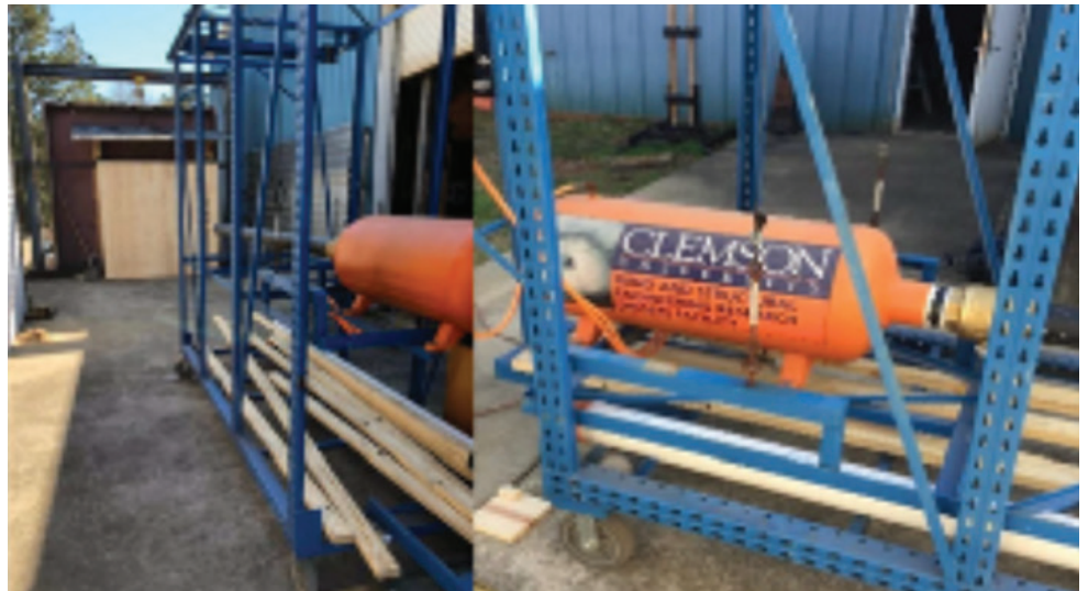
Figure 1. Pressure chamber for cyclic pressure/suction loading test
