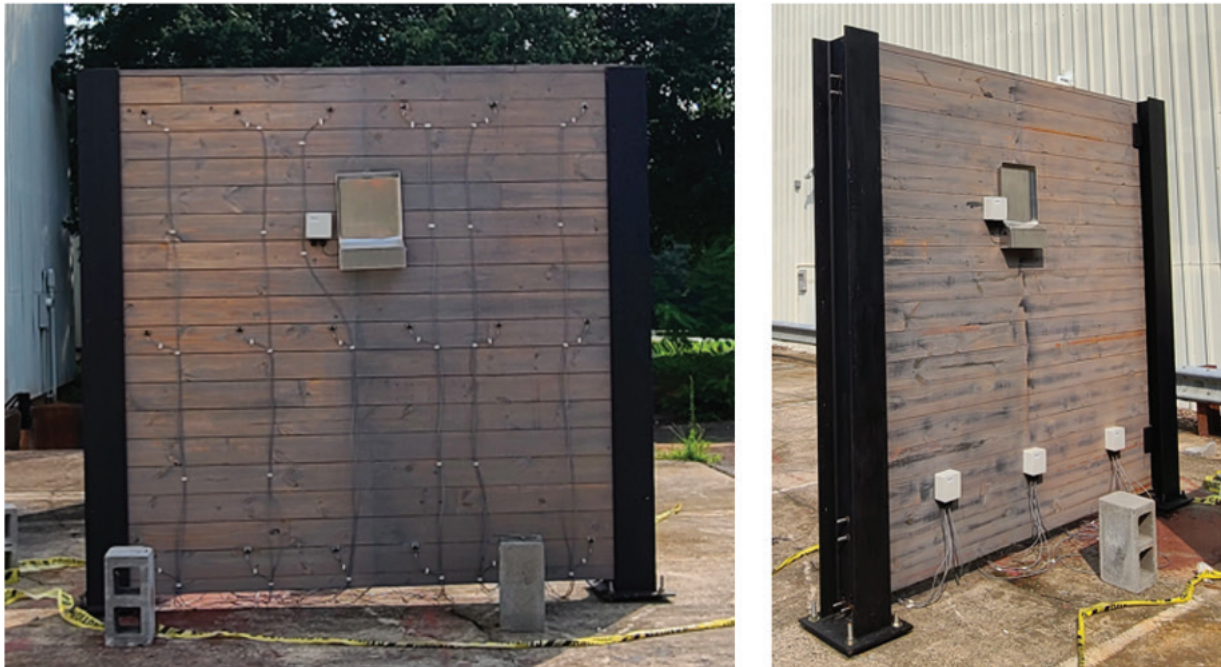
Figure 2: A mock-up construction of the proposed CLT noise barrier instrumented with moisture sensors and rain gauge for long-term moisture monitoring.
