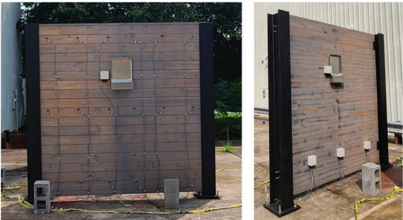
Figure 1: A mock-up construction of the proposed CLT noise barrier instrumented with moisture sensors and rain gauge for long-term moisture monitoring.
