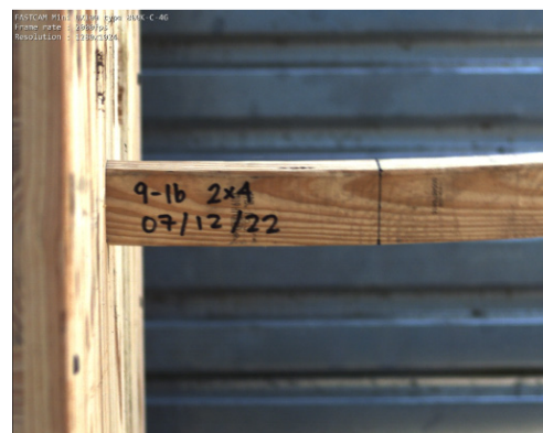
Figure 2. CLT specimen during the impact test.
