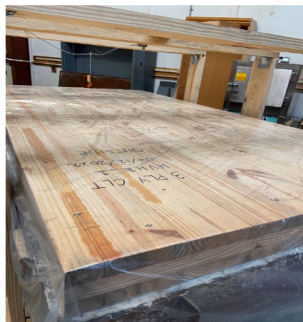
Figure 1. CLT specimen during the cyclic test.
