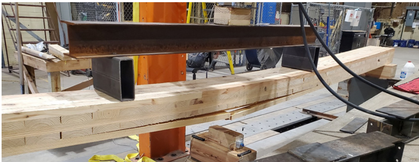
Figure 1: CLT bending specimen after failure
