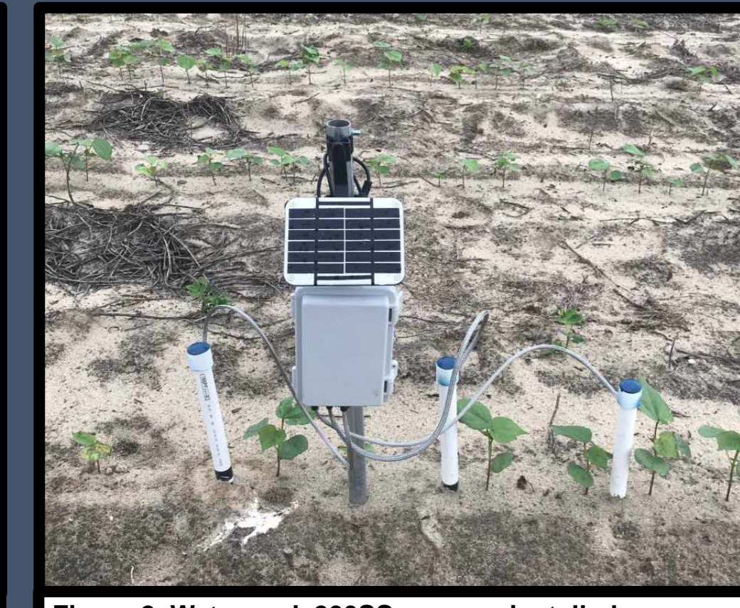
Figure 2. Watermark 200SS sensors installed.
