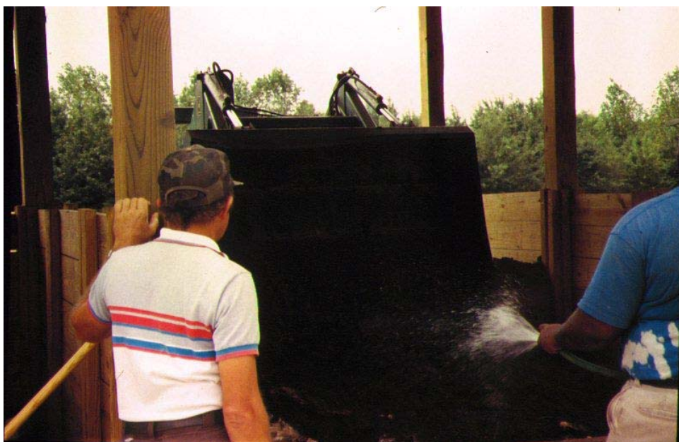
Figure 4.5. Aerating the composting material through mechanical lifting and dropping with a front-end loader and adding water to increase the moisture content during second stage composting.
