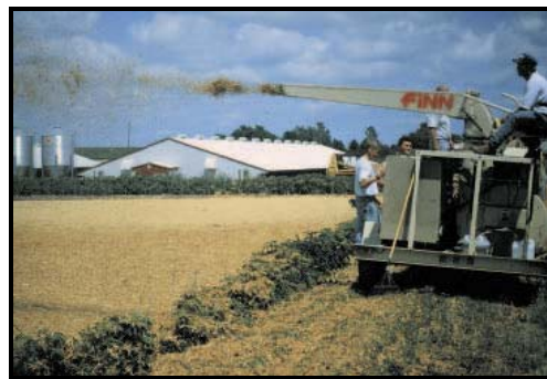
Figure 3. Blowing wheat straw onto a manure storage pond to form a biocover (Lorimar et al., 1998).
