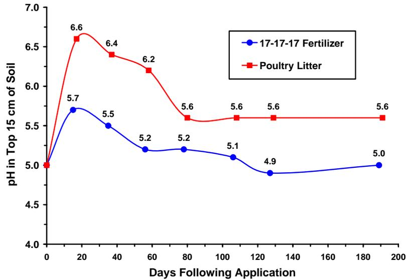
Figure 6. Affect of fertilization on soil pH.
