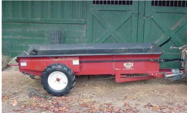
Figure 2. Small box spreader used to apply the turkey litter in the plot.
