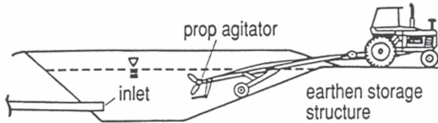
Figure 4.5. A propeller-type agitator (from the Liquid Manure Applications Design Manual, NRAES-89).
