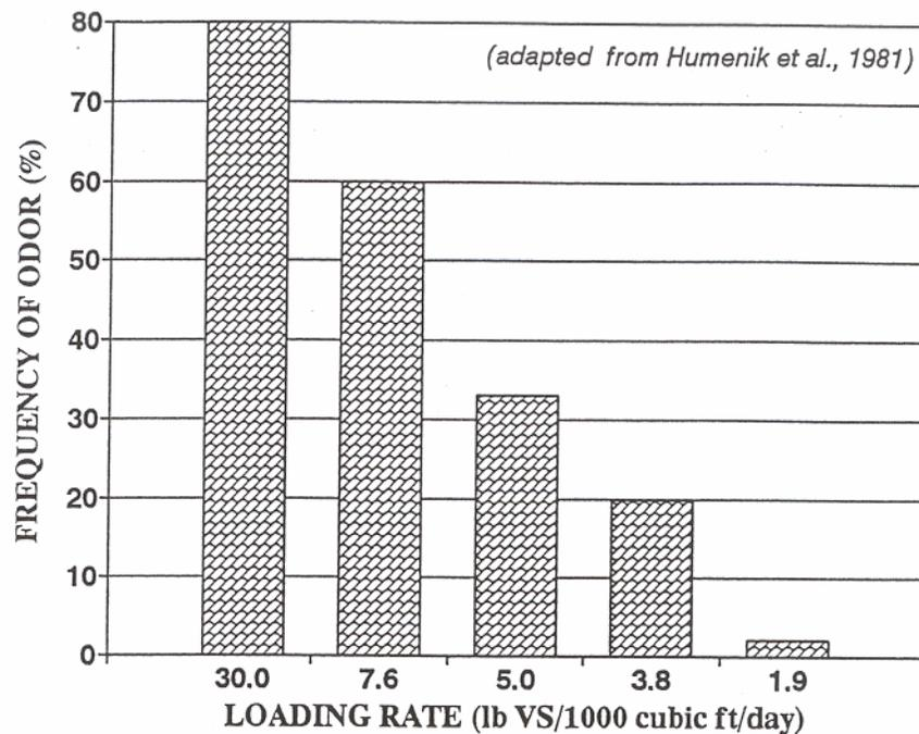
Figure 4.2. Effect of loading rate on odor production from lagoons and storages.
