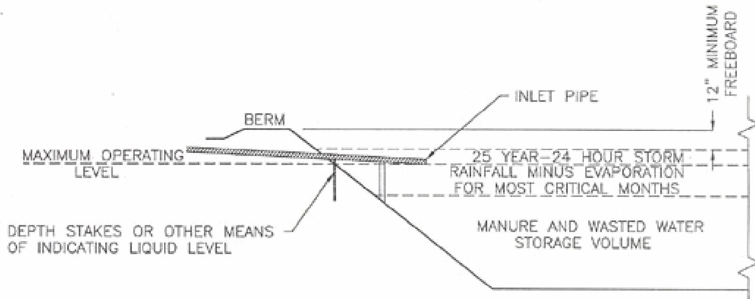
Figure 4.3. Components and Operating Levels for a Conventional Storage Pond
