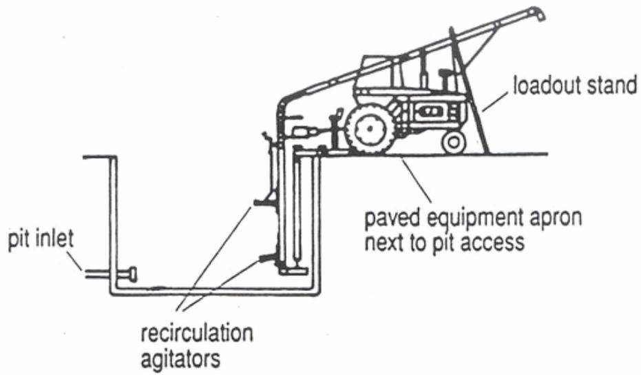
Figure 4.7. A below-ground storage tank (from Liquid Manure Application Systems Design Manual, NRAES-89).
