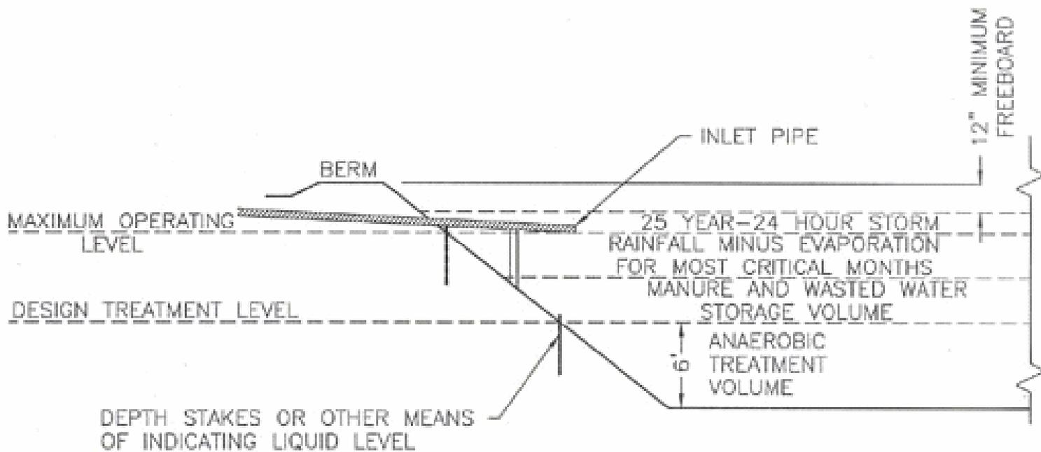
Figure 4.4. Components and operating levels for a liquid manure storage pond that includes a treatment volume for odor control.
