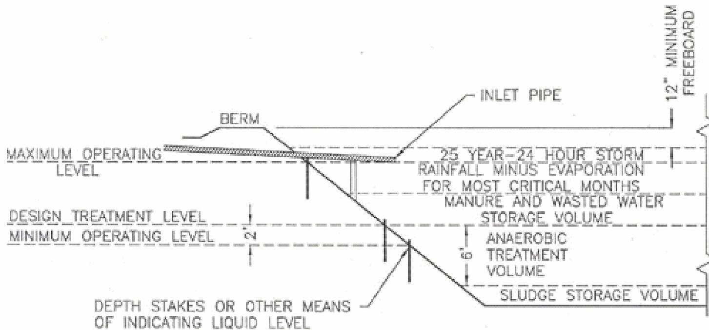
Figure 4.1. Components and operating levels for an anaerobic lagoon.
