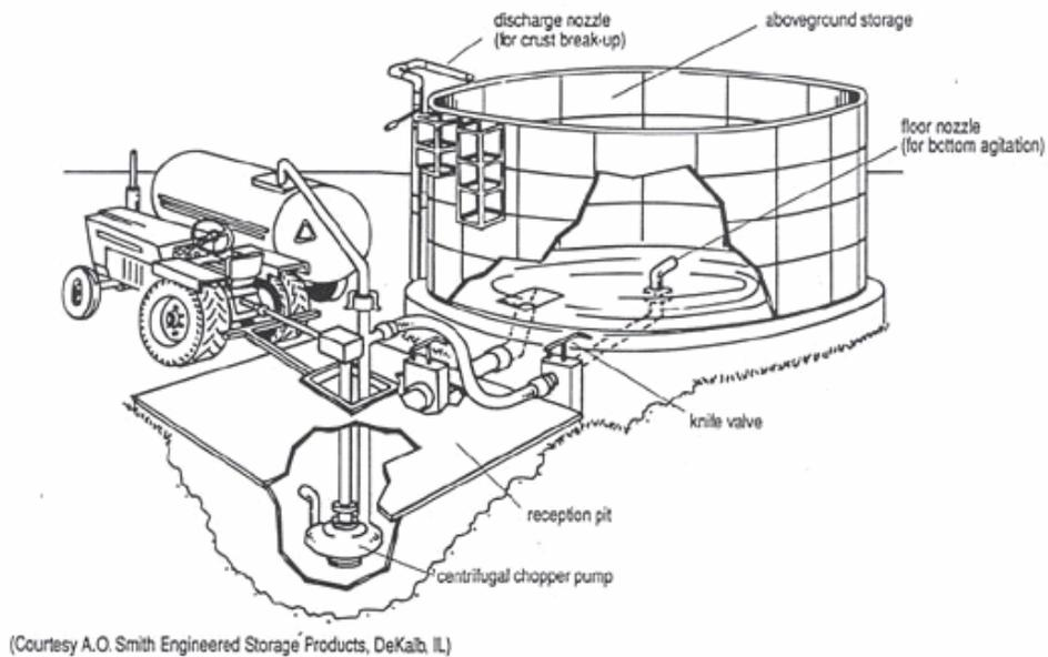
Figure 4.8. An above-ground storage tank and agitation system (from Liquid Manure Application Systems Design Manual, NRAES-89).
