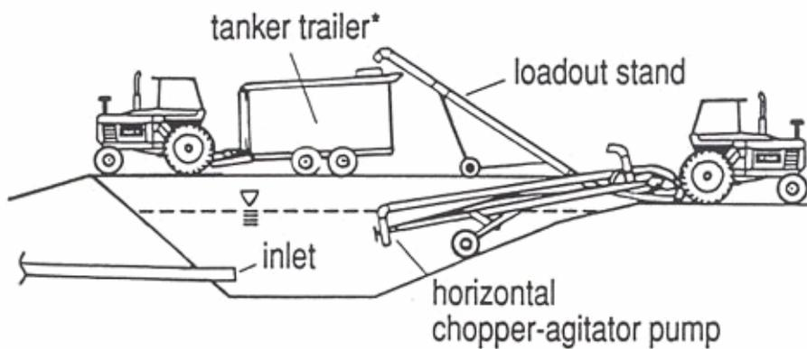
Figure 4.6. A centrifugal chopper-agitator pump (from the Liquid Manure Applications Design Manual, NRAES-89).
