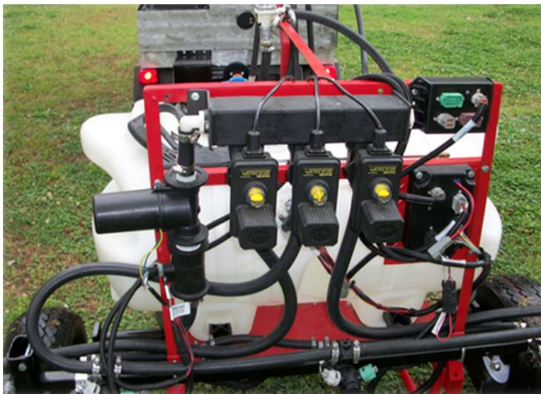
Figure 10. Controls for boom control and rate control.
