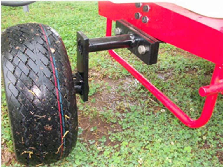
Figure 9. Axle pivot mount under the spray tank.
