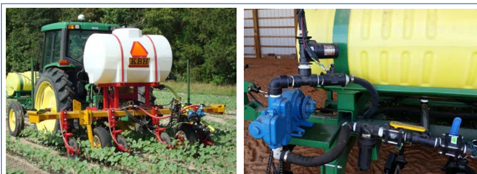
Figure 4: Clemson variable-rate nitrogen applicator with a Rawson controller (left), and the Southern Crop Solutions applicator (right)
