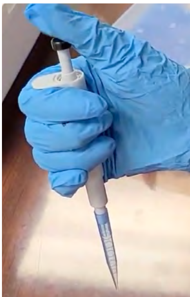
Practice finding the two pipette “stops” to collect and release sample water from the sterile tip (blue).
