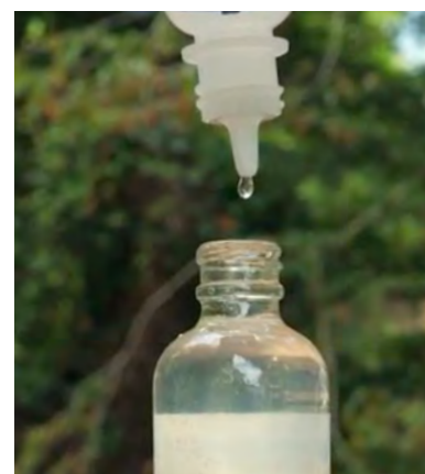
Hold the chemicals completely upside-down to maintain consistent drop size.
