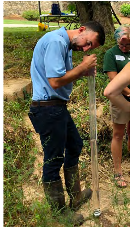
Look straight down into the tube while pushing down to release water from the base.
