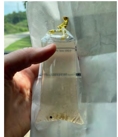
Discard and resample if sediment is stirred up and collected in the sample bag.
