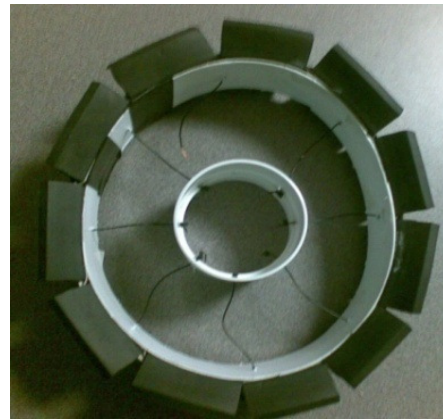
Plastic NPW Prototype for Traction Concept
