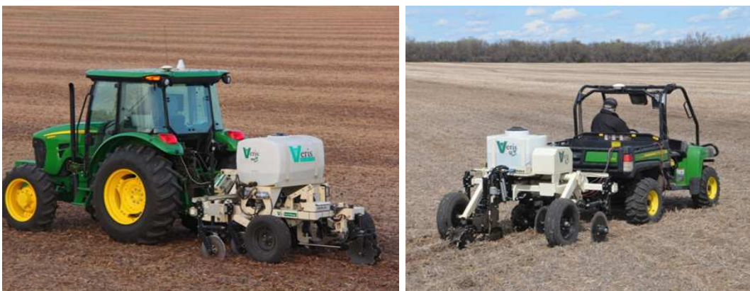
Veris MSP3 and U3 models that map soil EC, OM, and pH.
