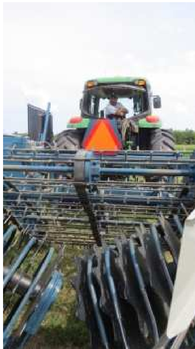
Clemson University agricultural engineer Kendall Kirk prepares to demonstrate a peanut digger that monitors and automatically adjusts blade depth to maximize yield.
