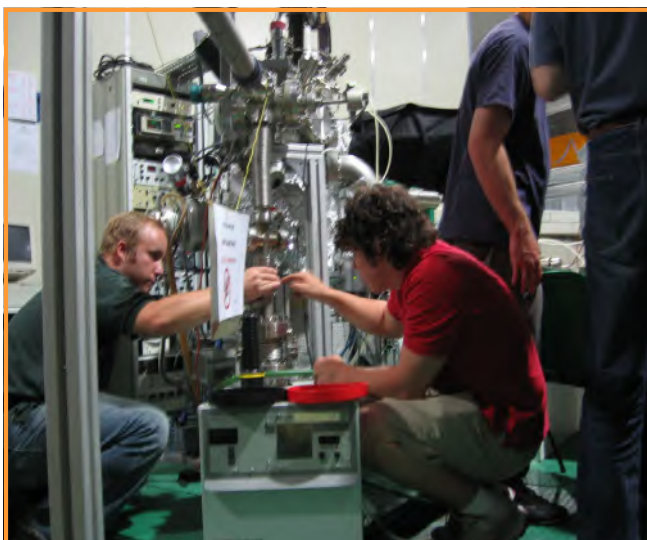
Matt Reaves (Univ. of Arkansas) and Tripp Collins (Clemson) prepare to insert a sample into the ultra-high vacuum chamber for analysis using XPS and LEED. This is one of the experimental stations at ELETTRA.
