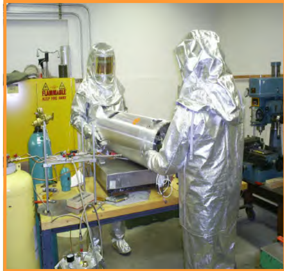
Loading TMA is one of the most hazardous duties that Shop workers must perform.
