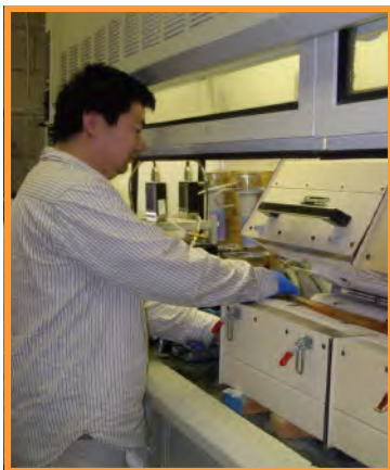
Carbon nanotubes are prepared by student, Keqin Yang, using a catalyst-assisted chemical vapor deposition method.
