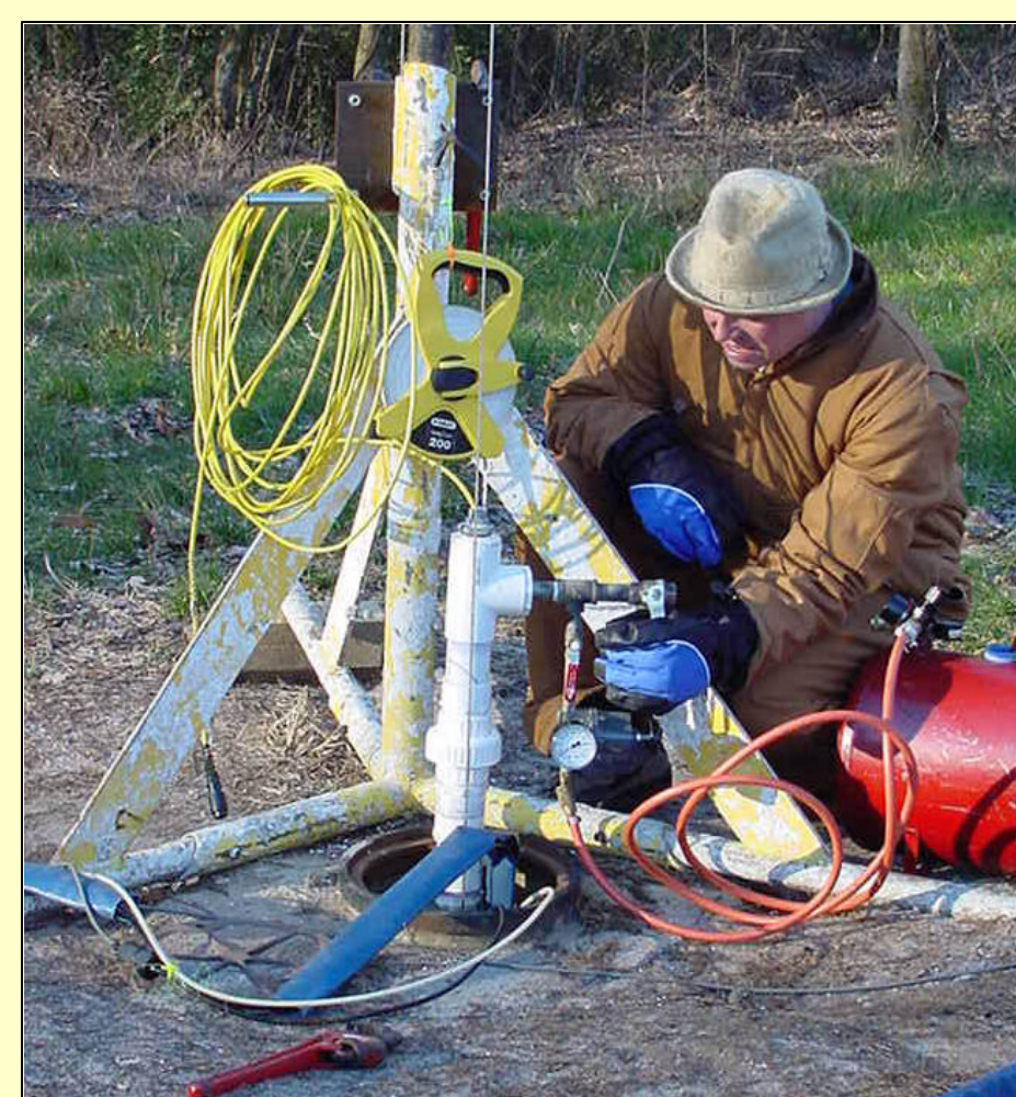
Above: Erik opens the valve on the well head to inject the air slug into the packed region.
