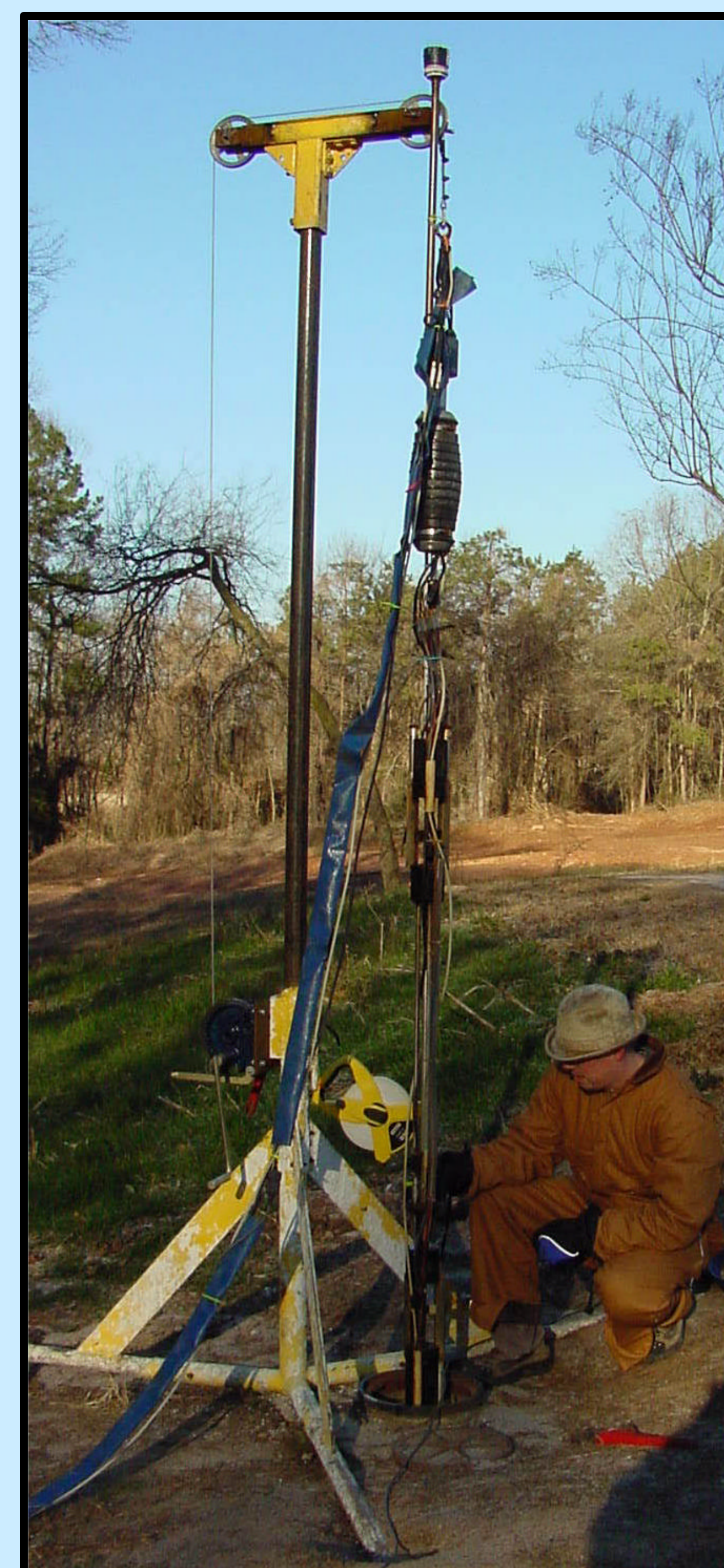
Above: Erik opens the valve on the well head to inject the air slug into the packed region.
