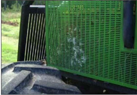
Cogongrass flower heads stuck in radiator grill. Photo by Mark Atwater, Weed Control Unlimited, Inc. Bugwood.org.
