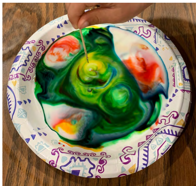
Figure 1. Active movement of liquid as surface tension is reduced.
