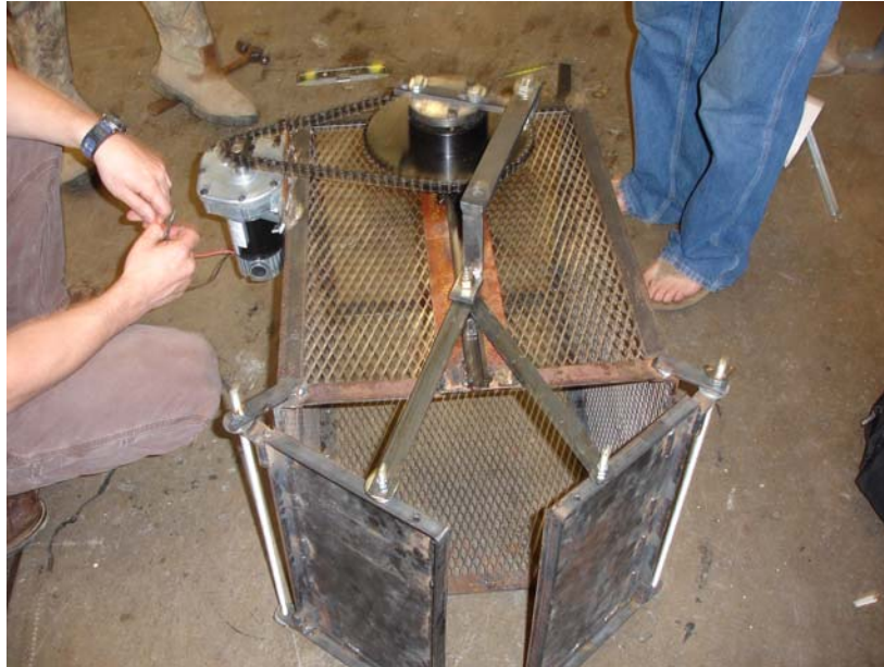
Figure 4. Trap doors on bottom of weighing bin, shown 75% open. Note: weighing bin is on its side in this image for testing purposes.
