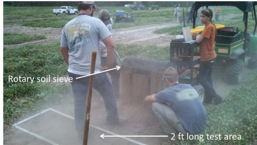
Figure 3. Digging loss sampling, showing excavated test area and soil sieve in operation.
