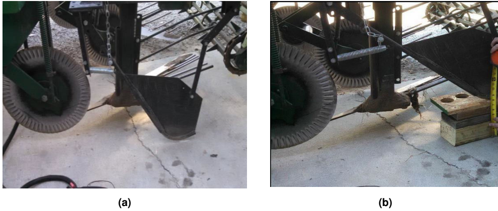
Figure 2. (a) The blade depth gauge trailed from the frame at the left side of the digger, and spring tension was provided to maintain contact with the ground. The rotary potentiometer was connected to the upper portion of the mechanical linkage. (b) Calibration of the depth gauge for linear measurement of blade elevation.
