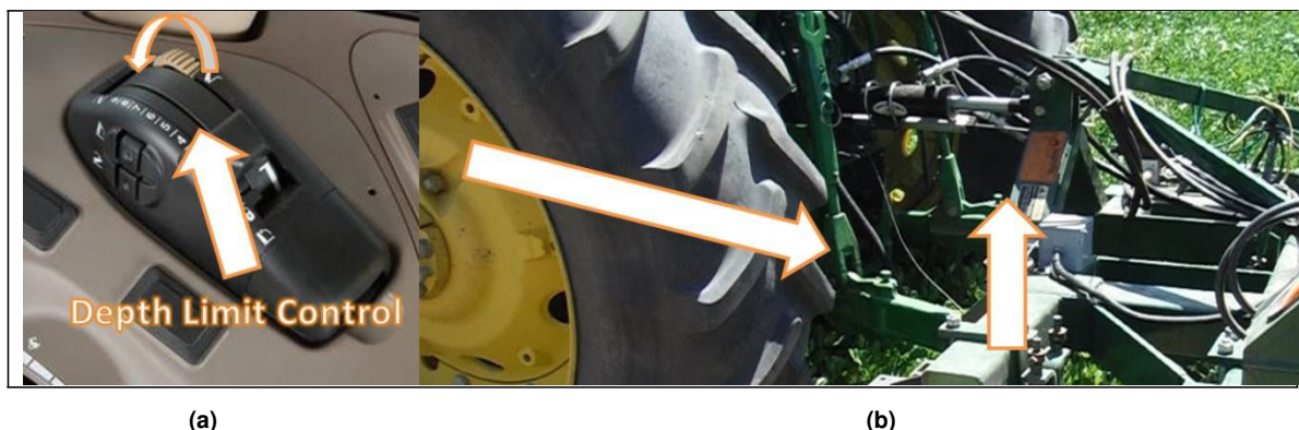
Figure 4. The depth limit control (a) used to adjust for the control-arm treatments. Two clicks were used for the depth limit in the medium EC zone, and four clicks were used in the low EC zone to raise the depth limit of the 3-point hitch lower control arms (b).
