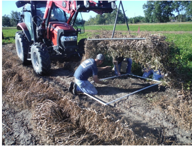
Figure 1. The custom made windrow lifter allowing individuals to remove above ground losses prior to combining.
