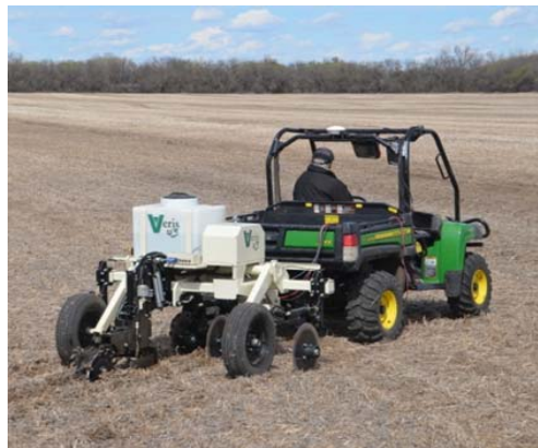
Veris MSP3 and U3 models that map soil EC, OM, and pH.
