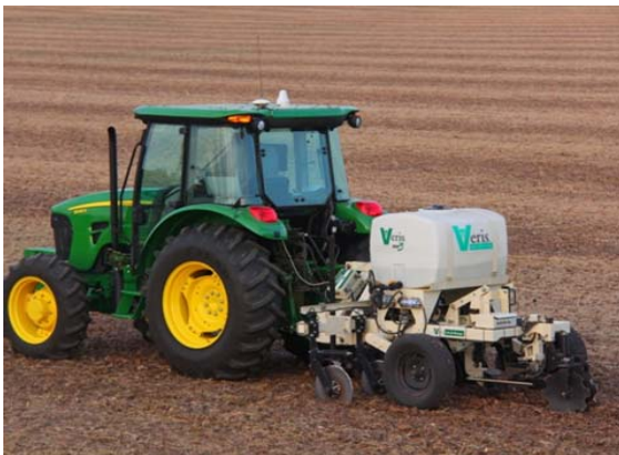
Veris MSP3 and U3 models that map soil EC, OM, and pH.
